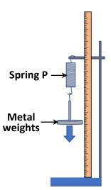
Forces were applied to the springs by attaching known weights. The extension of the springs was calculated for each force applied. The results are shown in the table.
